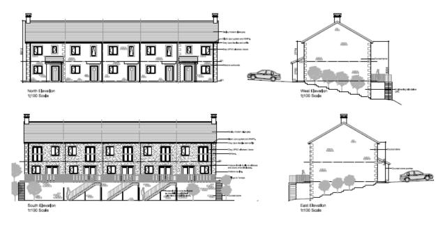
The proposed dwellings would be constructed in natural coursed stone to the front and sides and render to the rear elevation with slate grey coloured flat concrete tiles. Window and door surrounds and chimneys are used to reflect the character of surrounding terraces. The cross section below shows how the terrace would sit on the slope of the land with staircases to the rear to access rear gardens
